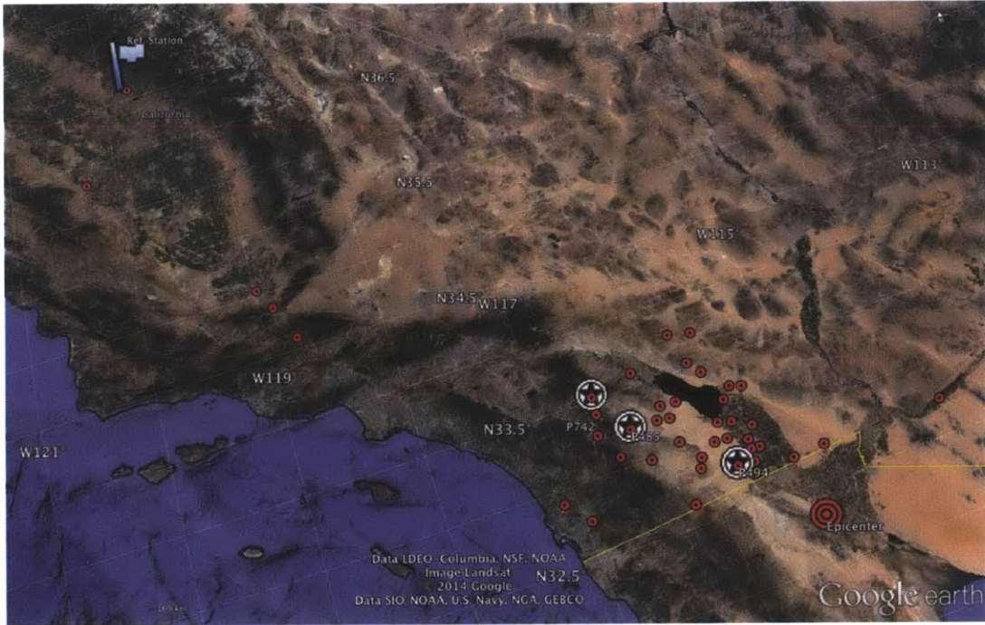
Figure 2-4: Map of GPS receivers used in this study. The station network is represented by small red targets. The earthquake epicenter is the large red target to the lower right of the image. The reference station is the white flag in the upper left corner, and the stations referenced in Figs. 2-5 through 2-8 are shown as white stars.
