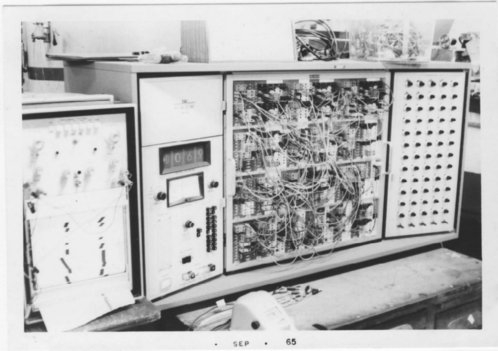
Hybrid computer, pilot control input recorder, gimbal power conditioner and controller.
