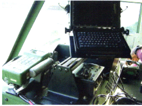
FIGURE 4.1: A mobile Army MTS computer system installed in a vehicle
