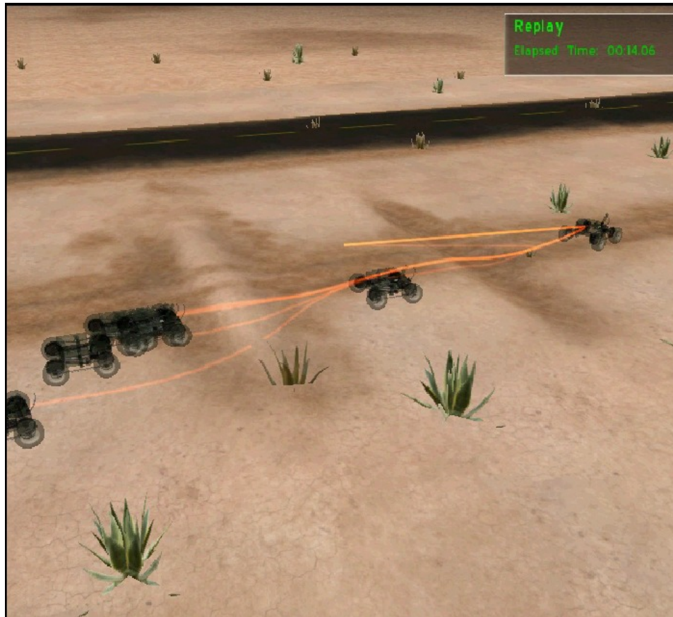
Figure 8: ANVEL Visualization Showing Repeated UGV Mobility Study. The "trails" show paths taken, with a UGV "ghost" remaining where the vehicle could progress no more given the particular constraints of that run.
