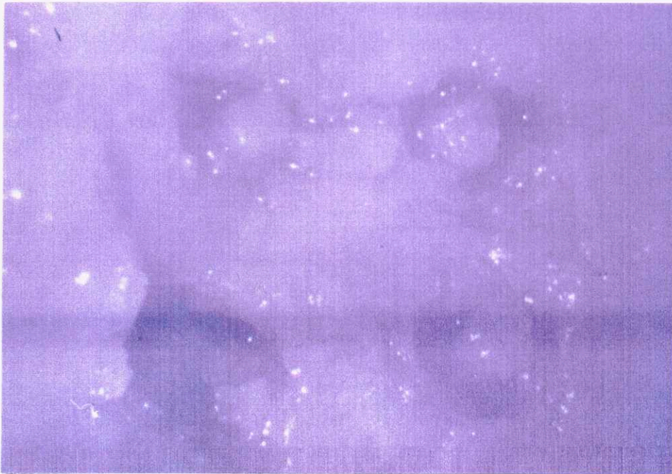
FIGURE 9.3. Full catheter craters in fibrous/fatty coronary artery. Ablation parameters: E_{\text{fiber}}(\text{bottom left crater}) = 15 \text{ mJ} , E_{\text{fiber}}(\text{other craters}) = 11 \text{ mJ} , n_{\text{fiber}} = 10 , m_{\text{round}} = 3 .
