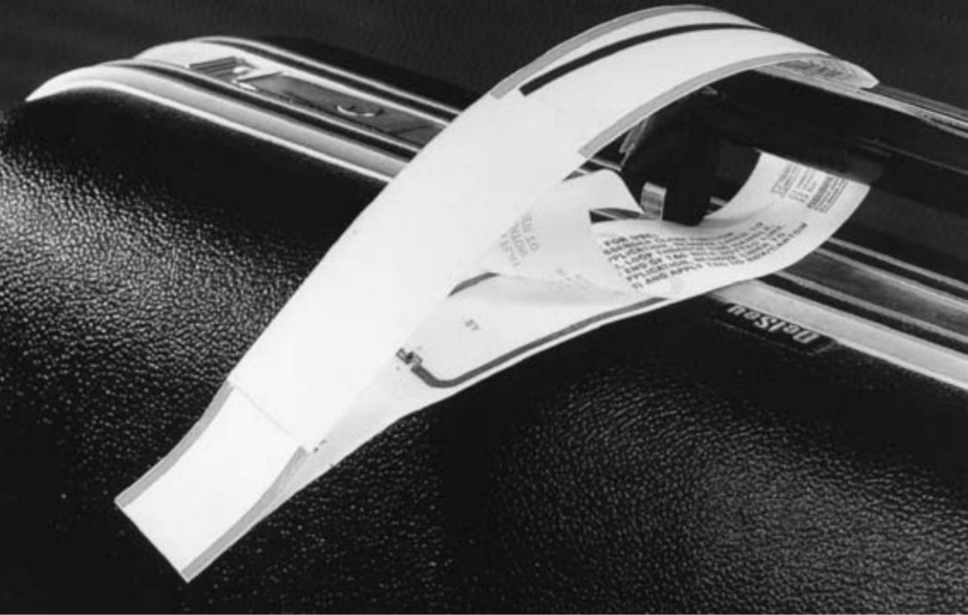
Smart label transponders are thin and flexible enough to be attached to luggage label (reproduced by permission of i-code-Transponder, Philips Semiconductors).
