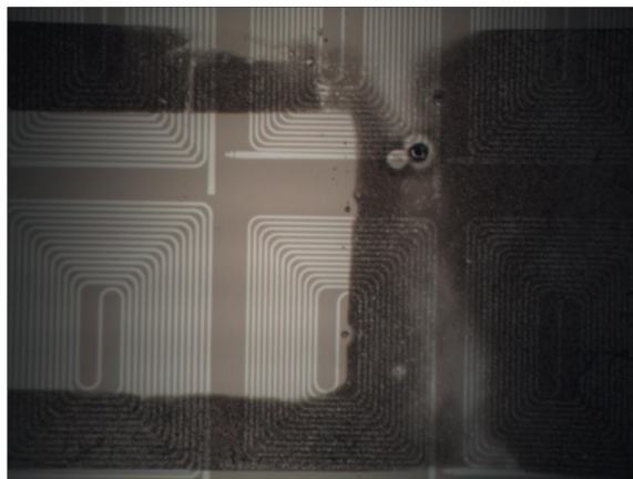
Figure 4.14: Resulting photoresist pattern due to over-development.
