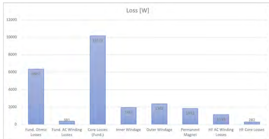
Fig. 2 Breakdown of electric machine loss
