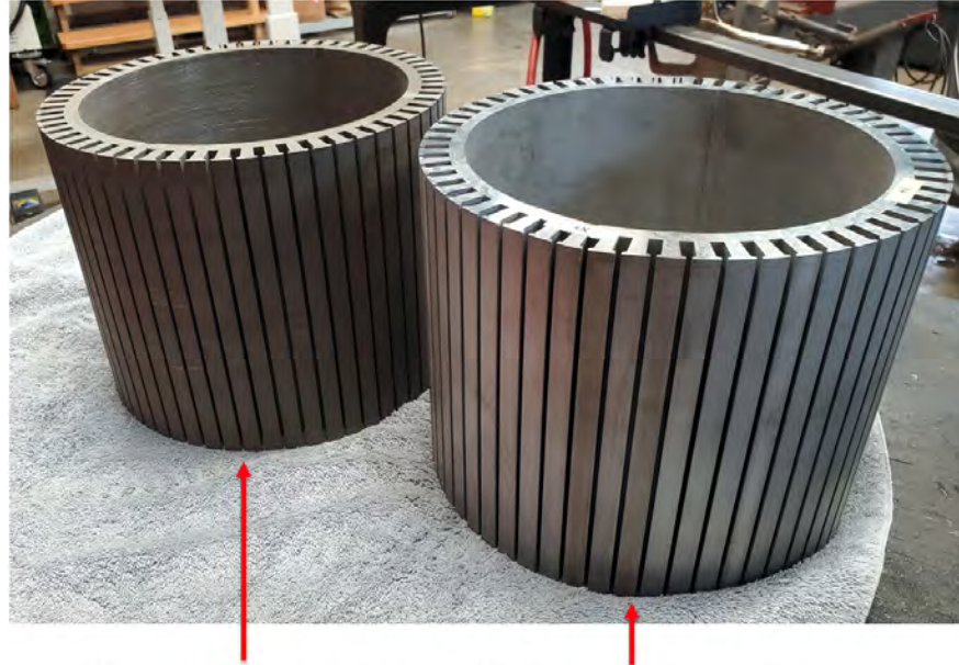
Process #1, Vacoflux 48 Process #2, Vacodur 49
