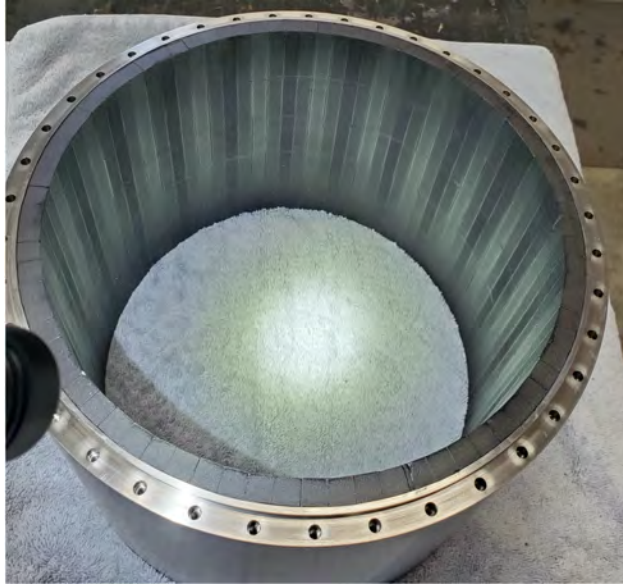
Fig. 19 Halbach array rotor was successfully manufactured
