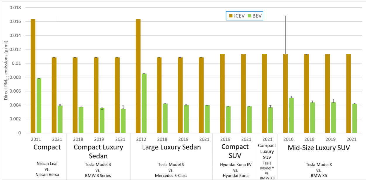
Figure A-22 - Combined cycle PM 2.5 emissions [g/mi] for vehicle type, size, model year, trim (bar=base, whisker=top) in MA
