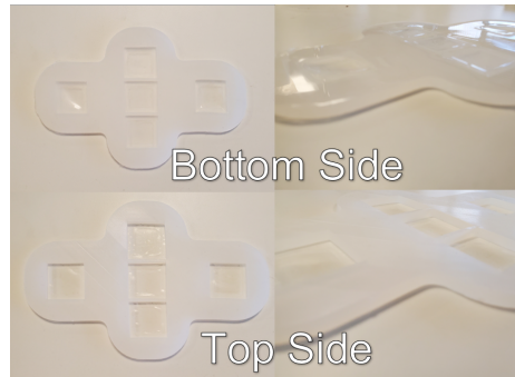
Figure 4-6: Silicone rubber conformable patch prior to the embedding of the transducers
