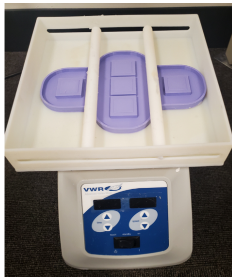
Figure 4-5: Mold fixed onto the shaker
