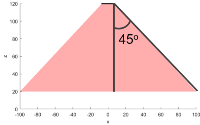
Figure 4-3: Definition of a transducer's FOV in the visualizer
