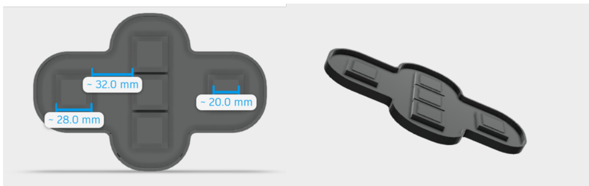
Figure 4-4: 3D rendering of patch mold
