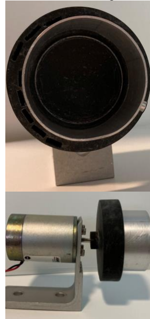
Fig. 5. Rotation Rate controller set. On the top Figure, we see the side view of the test setup. Here we see how the motor mount is attached to the motor shaft. The aluminium tube is also attached to the Motor Mount. The bottom image is the frontal view of the motor mount. On the bottom right, we can see the small magnet that has been placed in one of the side slots.
