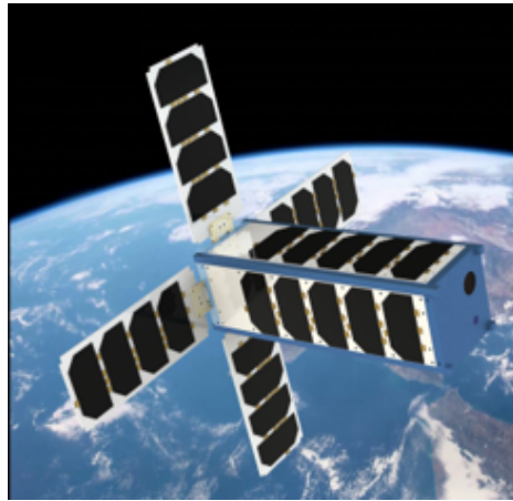
Figure 2-7: 3U CubeSat with deployable solar panels. Figure generated by Christian Haughwout [58].
