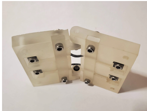
Figure 3-13: Buckling in each SMA's annealed direction.
