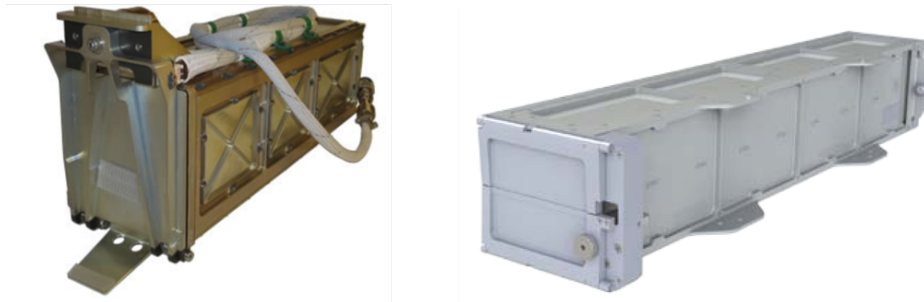
Figure 1-2: CubeSat dispensers. Left: P-POD CubeSat dispenser developed by Cal Poly. Right: NRCSD CubeSat dispenser developed by NanoRacks [8, 7].
