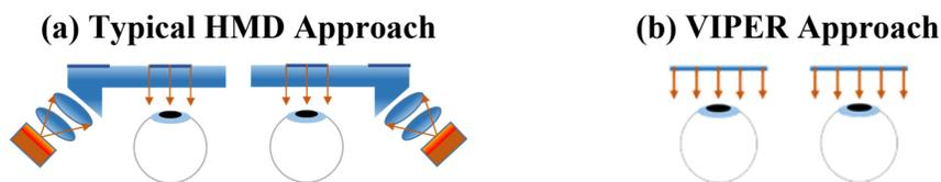
Figure 4.12: Simplified diagram of (a) a typical HMD approach using an optical relay system versus (b) the direct-view near-eye VIPER approach.
