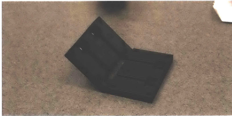
Figure 9. 3D-printed model of the version 1 hinge.
