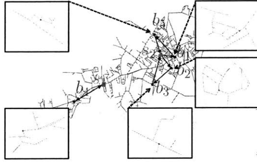
Figure 3-11: Optimal PIRP solution where all failures alerts occur one hour prior to t_0 . The arrows depict the routes for the inspection crews, which originate from the two service stations (triangles) and visit the temporary bases within each subnetwork
