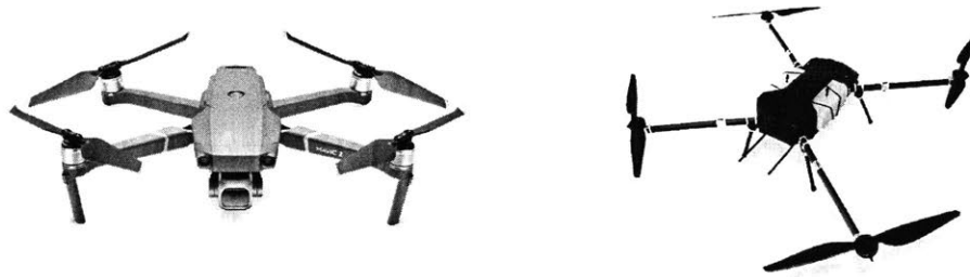
(a) Example of Shorter Endurance UAS: DJI Mavic Pro (b) Example of Longer Endurance Hybrid UAS: Skyfront Perimeter
