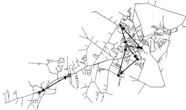
Figure 2-3: Illustration of inspection crew tours. Starting from a service station, each crew visits one or more temporary bases (black dots) and returns to its station (triangles)
