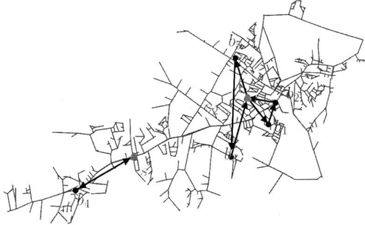
Figure 3-12: Optimal PIRP solution for the case where the failure alert for subnetwork 2 (resp. 5) occurs 5 (resp. 3) hours prior to inspection crew dispatch
