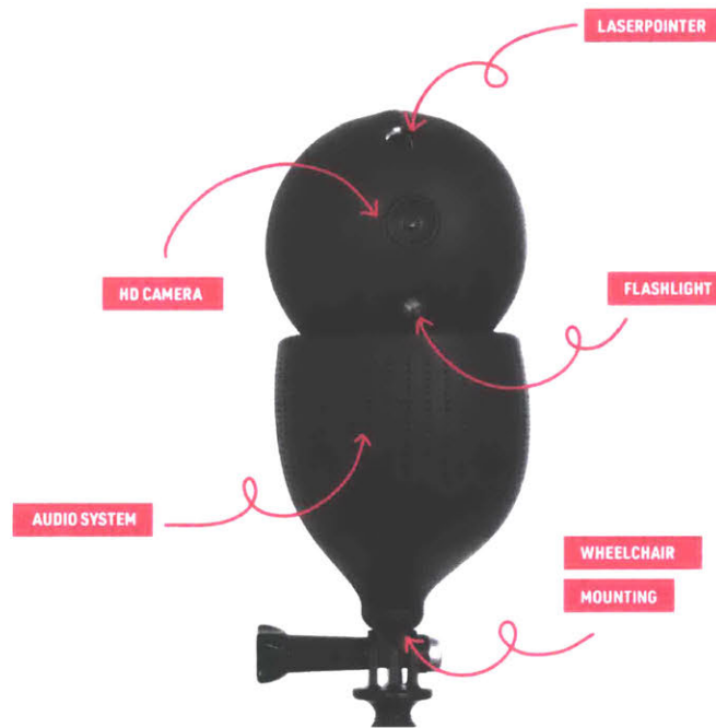
Figure 30: Loro's Companion Robot for Wheelchair Users
