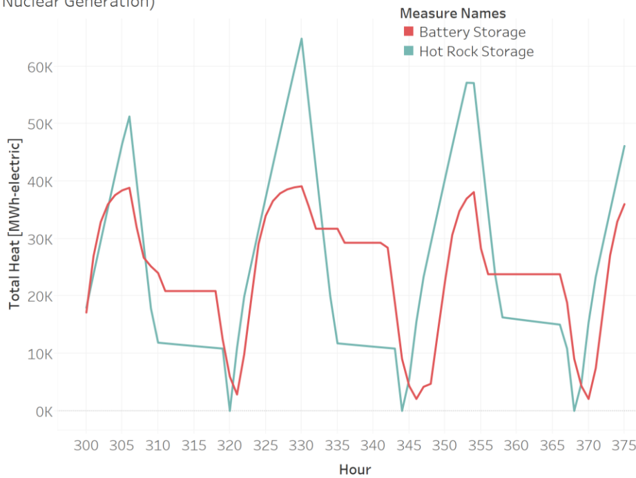
Storage Levels for Favorable Case with $1/kWh and 5 g CO 2 /kWh (43 GWe Coupled Nuclear Generation)
