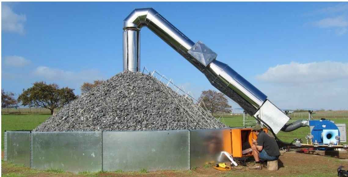
Figure 13 – STERG Group Experimental Rock Bed (Laubscher SolarPACES)
