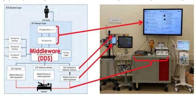
Fig 5: General architecture of ICE and an instantiation of it in a test setup at MD PnP Lab
