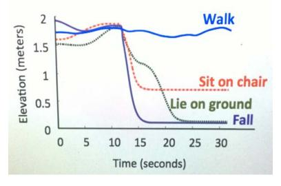
Fig 4: Predict the possibility of fall by analyzing the data from reflected radio waves [55]
