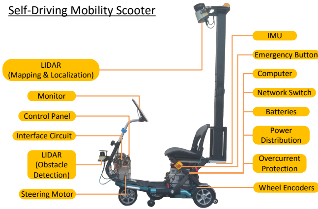
Fig. 1. Hardware overview, highlighting primary retrofit additions to a personal mobility scooter in order to enable autonomous capability
