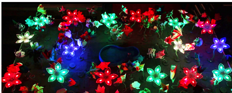
Figure 7.14: The garden can effectively demonstrate graph coloring algorithms. The tiles communicate with each other to determine a coloring such that no two adjacent nodes, including diagonals, have the same color.
