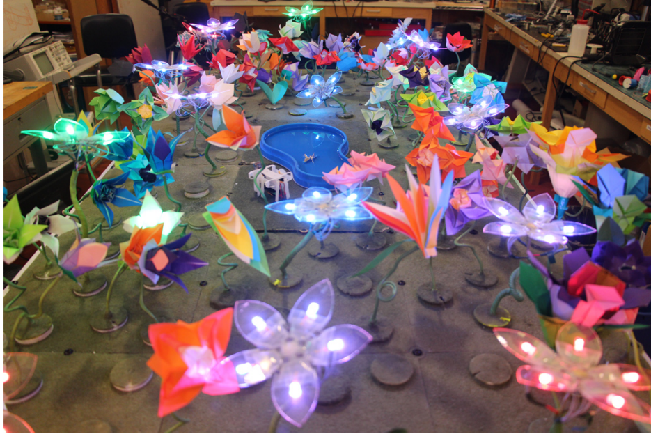
Figure 7.10: The distributed robot garden provides an aesthetic platform for teaching robotics and engineering or demonstrating computer science algorithms. It features nearly 100 origami flowers that can open and close, many of which can also light up and change color.
