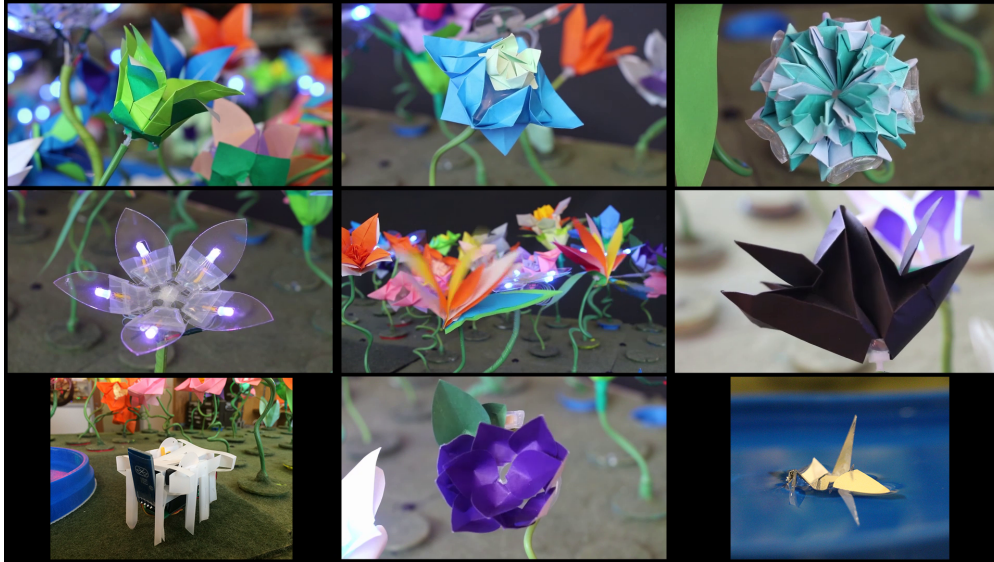
Figure 7.11: There are multiple types of flowers in the garden, which are pneumatically actuated to open close. There are also hexapod walkers (lower left), and a swimming crane (lower right).
