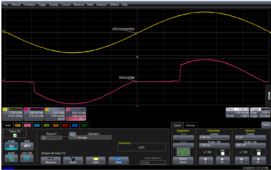
Figure 7-2: Oscilloscope voltage traces for an I_c sweeping measurement. Shown in yellow is the sine-wave reference voltage produced by the AWG. In pink is the voltage of the device under test (in this case an SNSPD).
