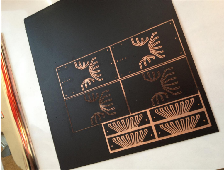
Figure 7-13: The laser-patterned PCB, parts of which have been cleaned with a Q-tip soaked in isopropyl alcohol. Before etching, the entire pattern should be as shiny as the original bare copper was before spraypaint application.
