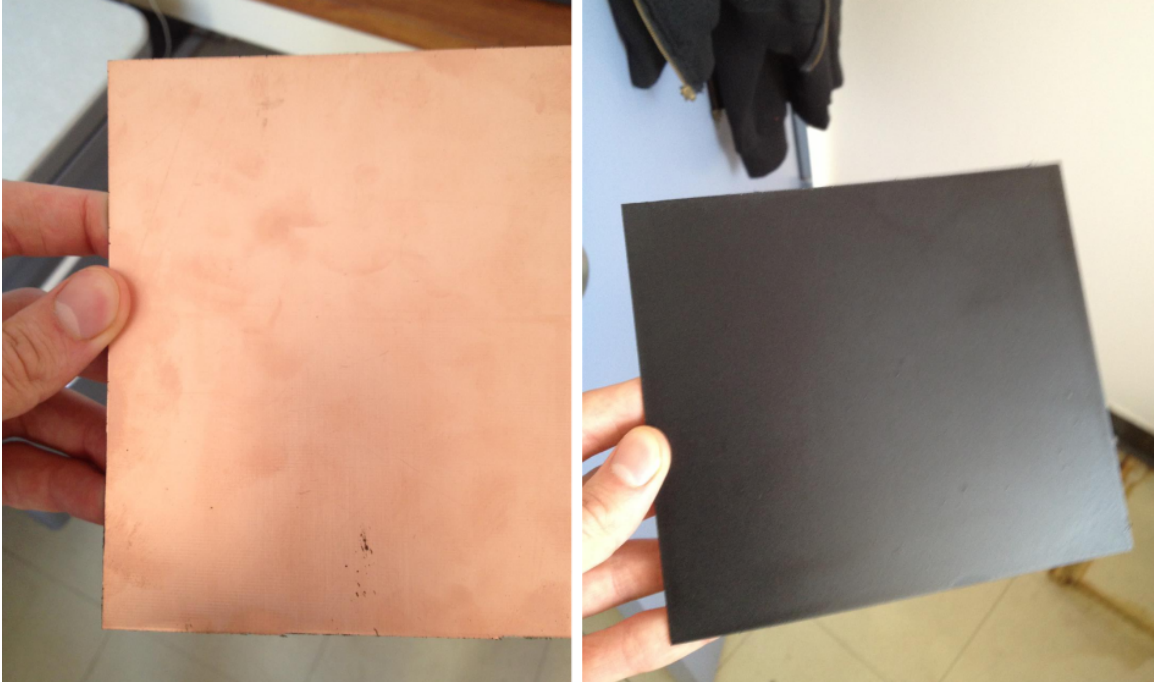
Figure 7-10: (left) Bare copper PCB board used as the blank substrate for PCB patterning. (right) The same copper PCB board, covered with two coats of black spraypaint.
