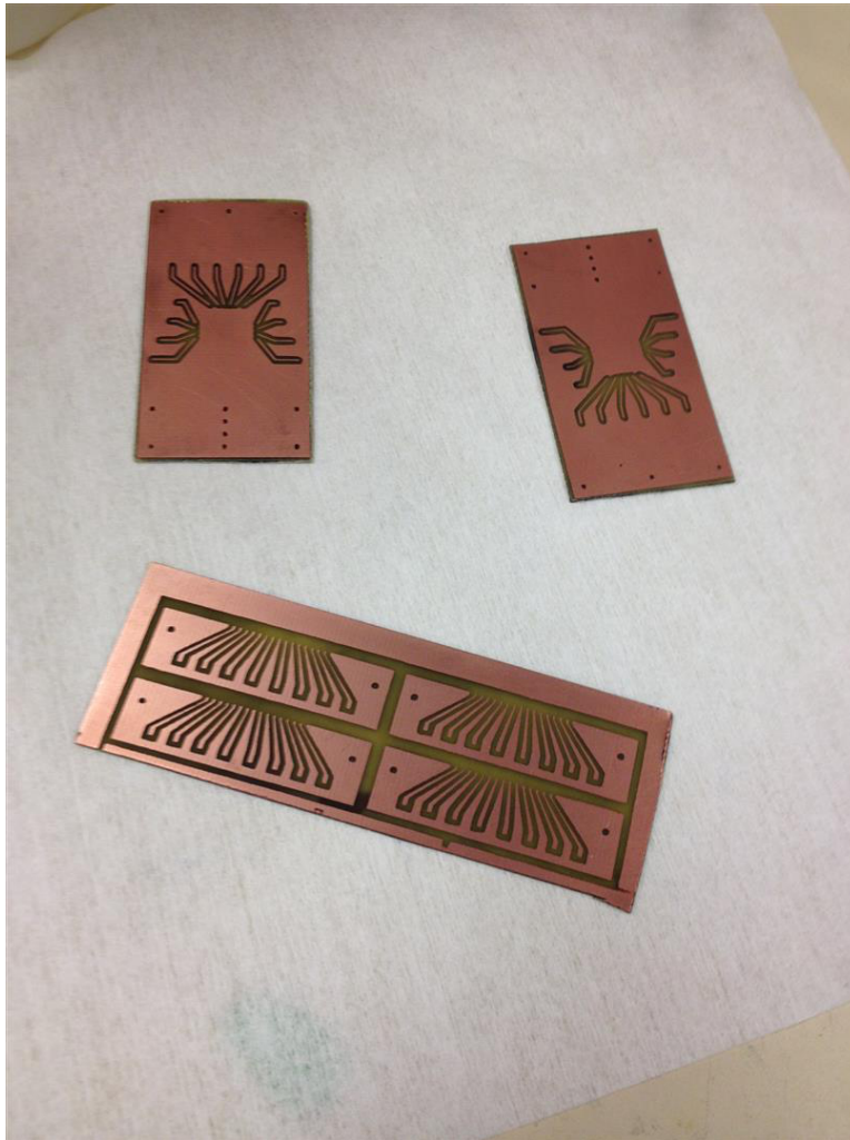
Figure 7-14: The final product from the in-house PCB fabrication process using the laser cutter.
