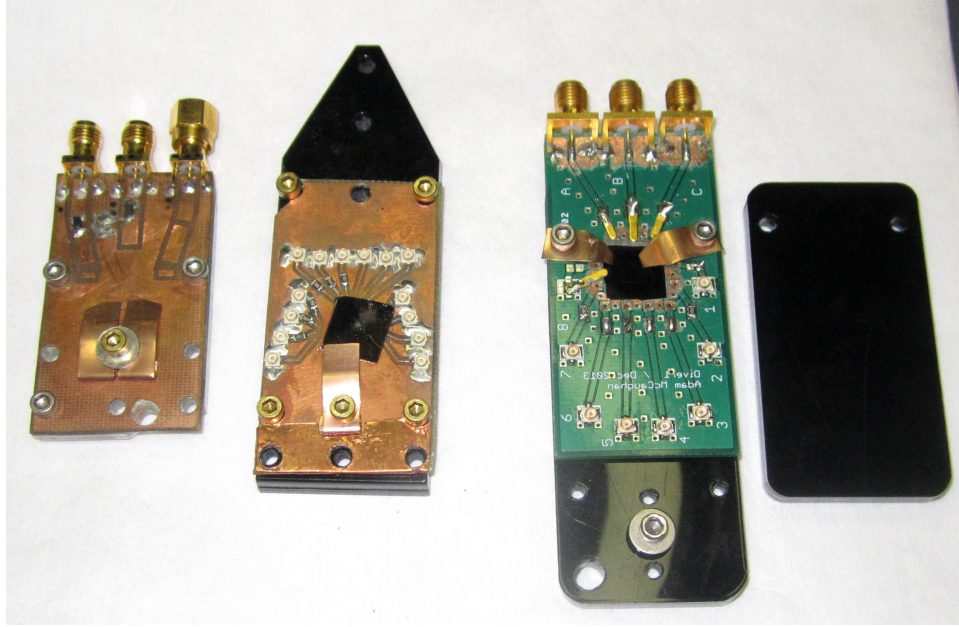
Figure 7-6: Photograph of three different custom-built sample holders. The two sample holders on the left were constructed from PCBs that were fabricated in-house using the etching process described in this thesis. The other sample holder (green PCB) had a PCB which was designed in-house but purchased from a commercial PCB company.
