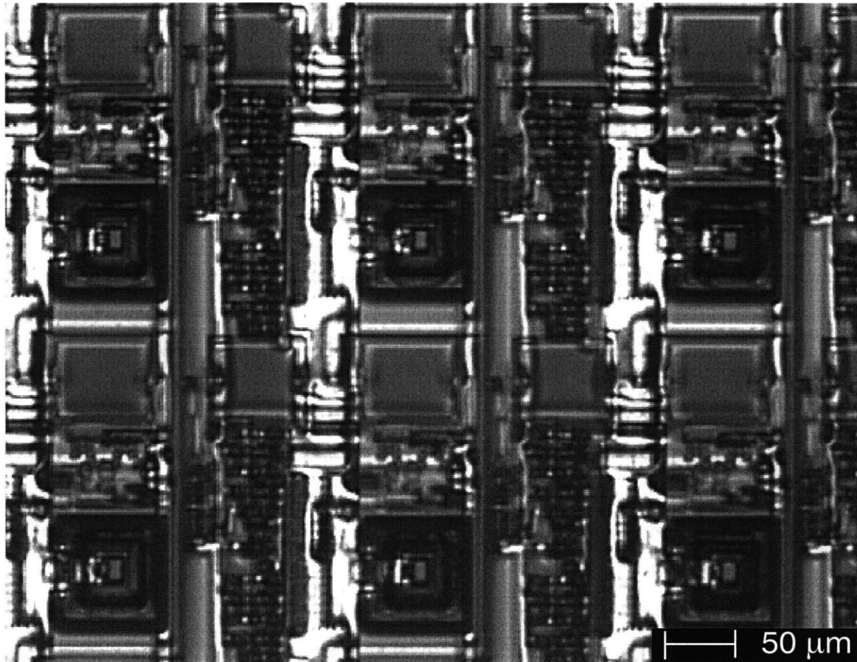
Figure 2.28: Integrated LEDs, MSM photodetectors, and VLSI electronics
